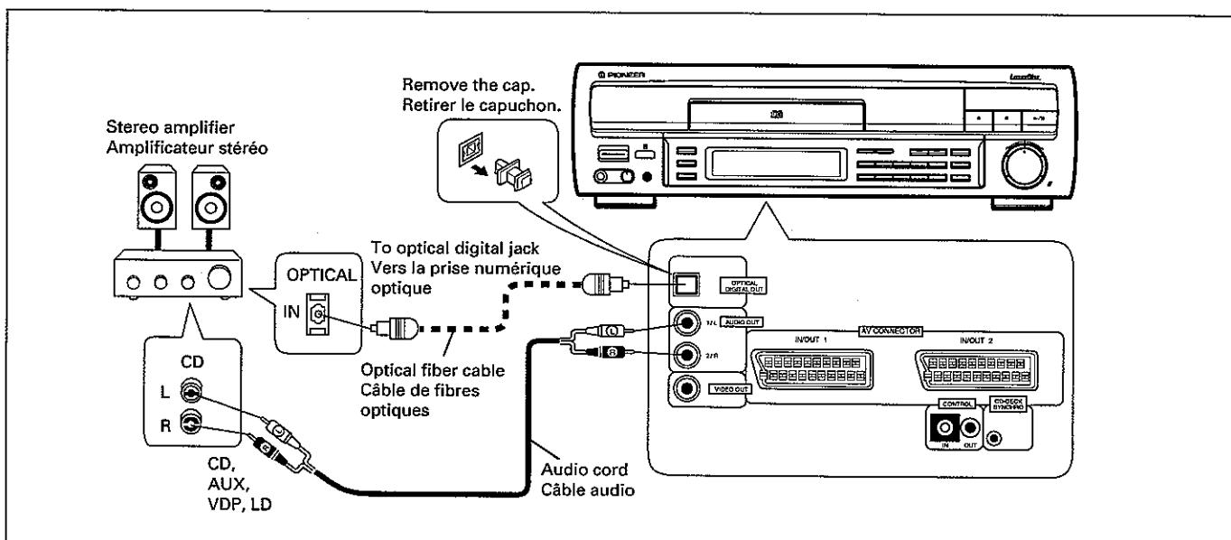
Connect the AUDIO OUT jacks of the player to the AUX, CD, LD or VDP input jacks of your stereo amplifier.
