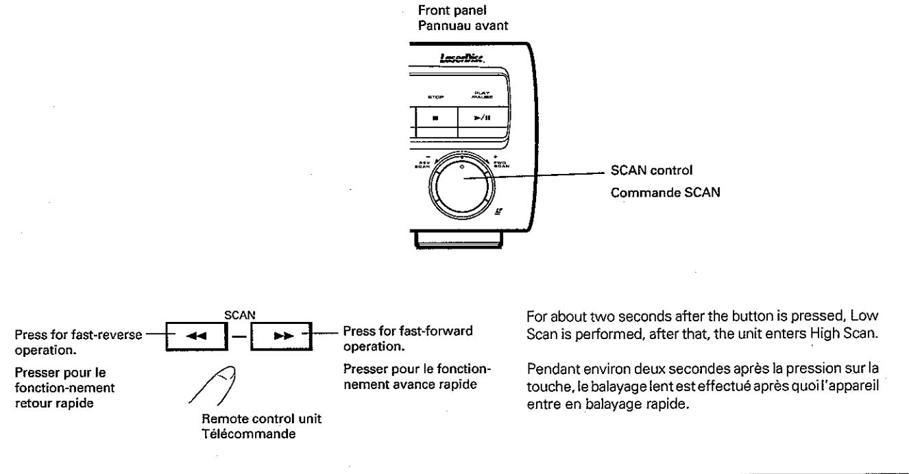
While rotating the SCAN control, playback advances or reverses at high speed. There are two scan modes which can be selected with rotational angles of the control.
