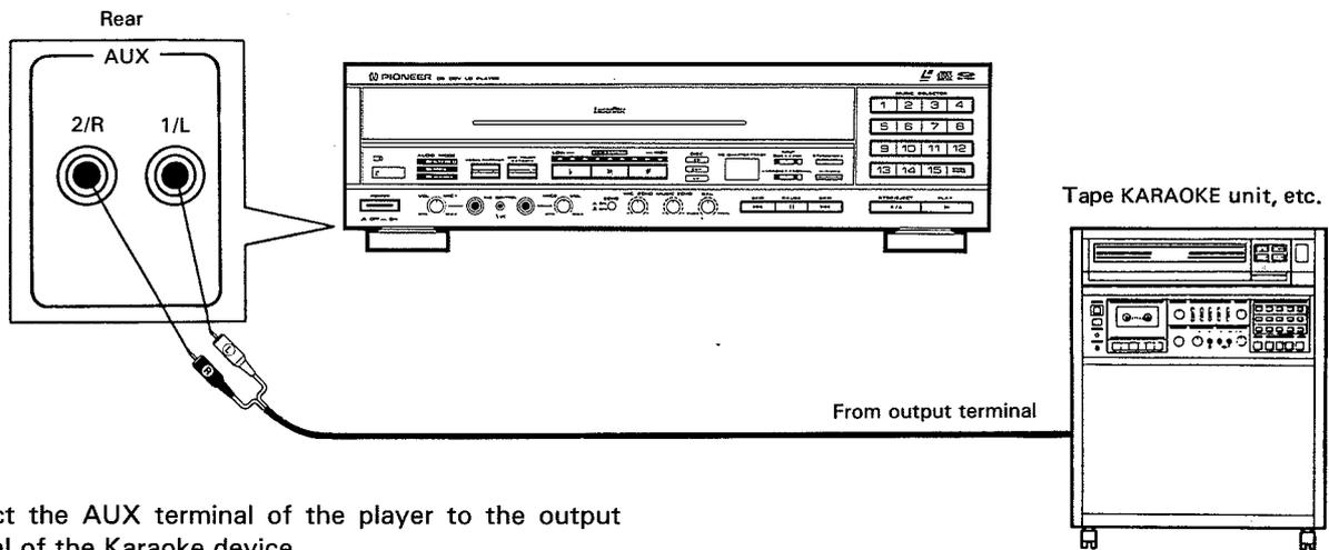
Connect the AUX terminal of the player to the output terminal of the Karaoke device.
