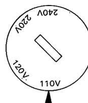
Set the selector so that the arrow points power voltage of your area (Figure shows arrow pointing to 110 volts.)
