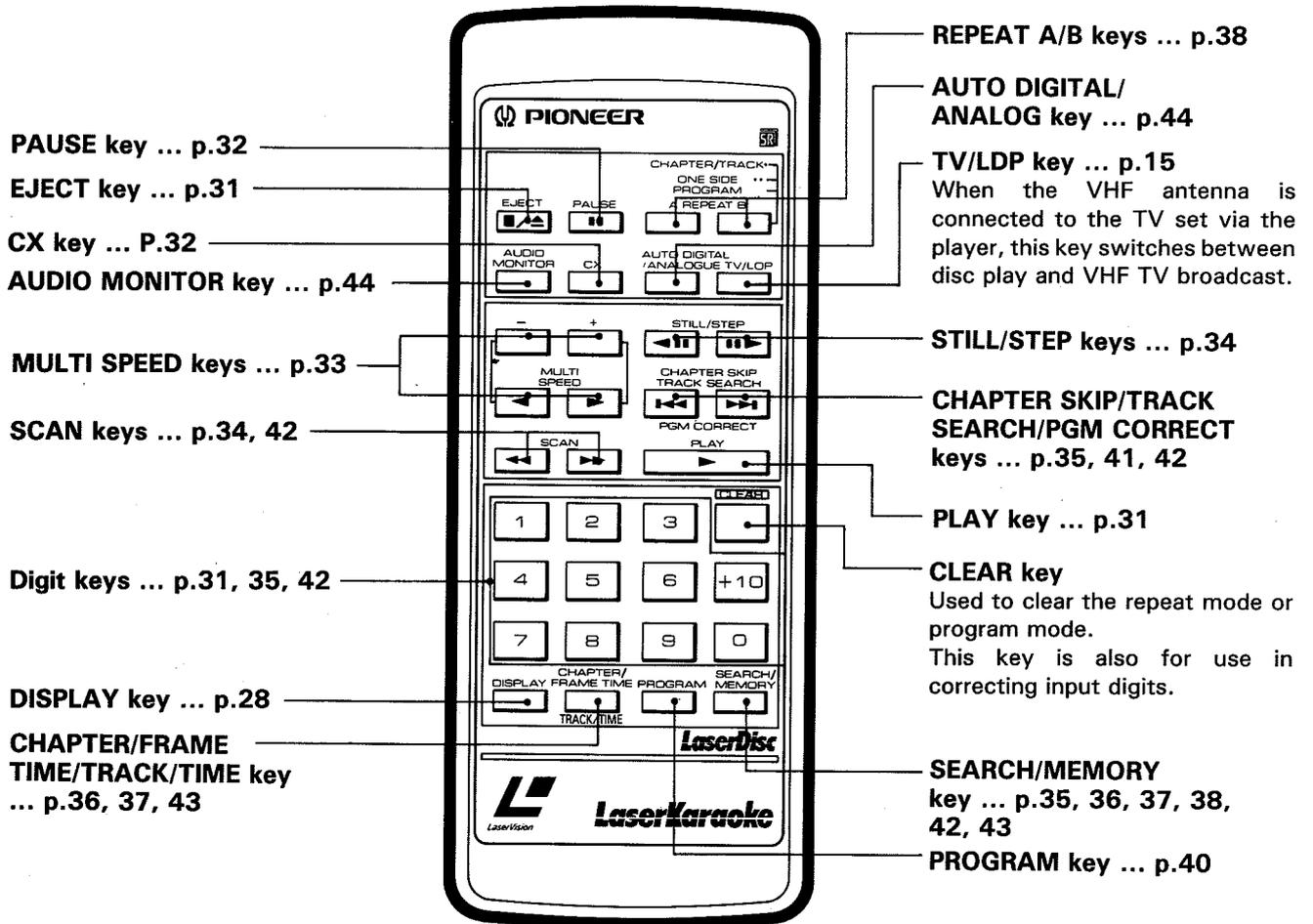
The illustration shows the remote control unit for the CLD-V700.
