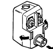
Pry open both latches and remove the cover.
