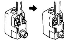
Loosen the screws, twist the wire around and tighten the screws.
