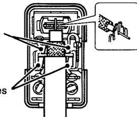
Tighten both sides with pliers.
